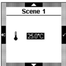
If temperature is selected, it is necessary to set next the temperature value desired using button **▲** and **▼**.
