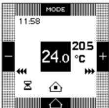
Pressing the button repeatedly allows to switch to Comfort mode for a limited time period.
